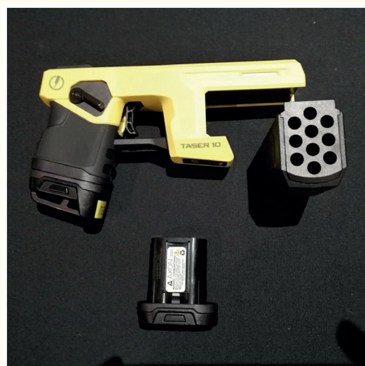
Axon's latest PESW model, the TASER 10, which, unlike its previous models, does not have the “drive stun” mode © Omega Research Foundation
